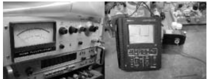
FIGURE 2 (left) Keithley electrometer used in tests. The sensitivity of this instrument allowed critical measurements. (right) Tektronix TDS 710 scope hooked to RF current transformer placed in the Tesla coil's primary circuit.
