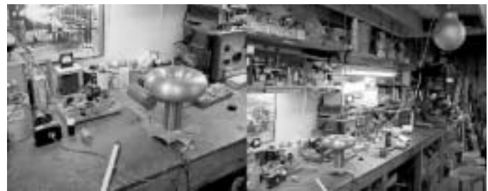
FIGURE 1 (left) Basic Tesla coil system with pulser system and (right) overall view of transmitter and receiver. The distance between the toroid and the sphere was 145 cm.
